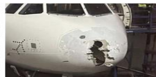
The IndiGo aircraft's nose cone was damaged in the turbulence, leading to its grounding for inspection and maintenance. (PI)
