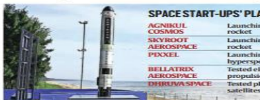
Agnibaan SoT-ED by Agnikul Cosmos is a 3D-printed suborbital rocket. X/AgnikulCosmos
