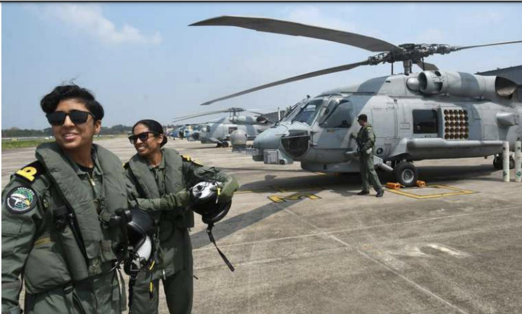
Latest addition: The Navy's newly inducted MH 60R Seahawk multi-role helicopters seen at INS Garuda in Kochi on Thursday. The Navy is set to commission MH 60R, which is capable of firing torpedoes, missiles and Advance Precision Kill Weapon System rockets. The self-protection suite on the helicopter comprises chaff and infrared flares, which can be deployed automatically upon detection of threat. THULASI KAKKAT
