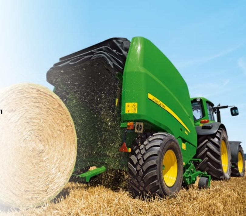
Before using a baler machine, farmers cut the crop residue with a tractor-mounted cutter. A tractormounted baler machine compresses the stubble into compact bales using netting.
